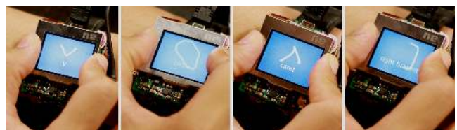
Figure 8. Gestures can be input by clicking and panning.
