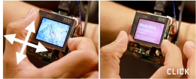
Figure 3. Panning the watch moves the map, twisting zooms in and out, and clicking shows details.
