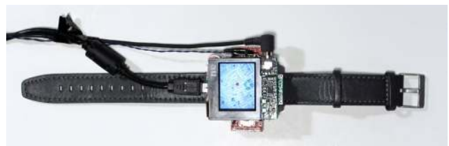
Figure 2. Our prototype uses a pair of Hall-effect joystick sensors, providing a multi-degree-of-freedom interface.
