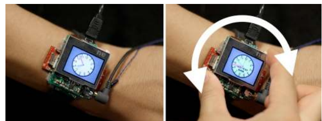
Figure 4. Clicking and then twisting sets the alarm time.
