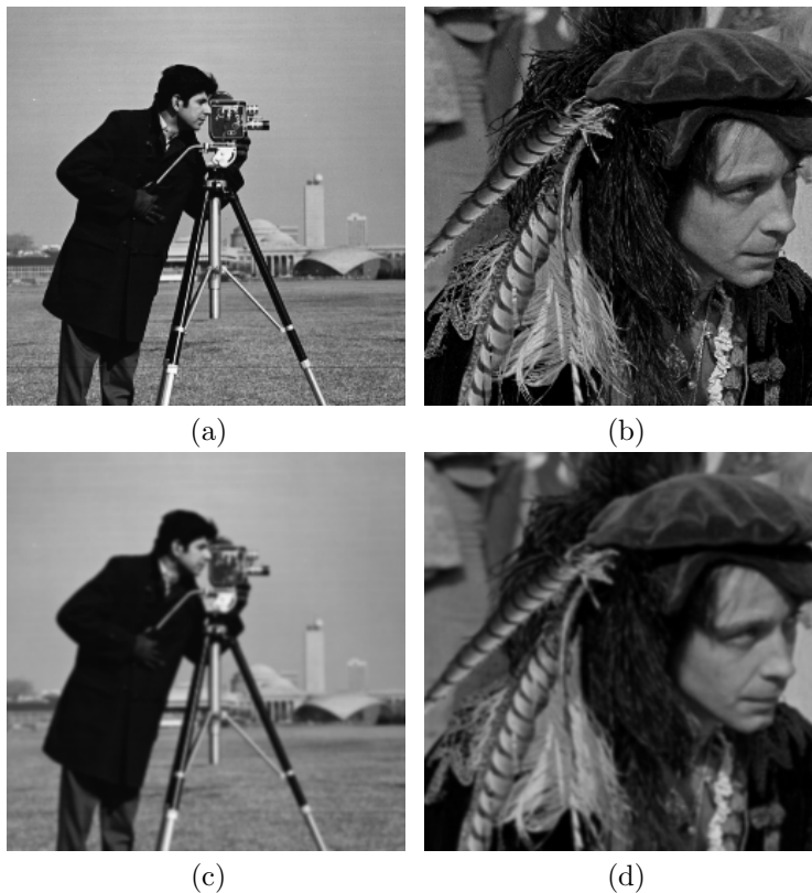
FIGURE 2. (a) Cameraman, (b) Man, (c) Cameraman with Gaussian convolution with a 9-by-9 window, (d) Man with Gaussian convolution with a 9-by-9 window.
