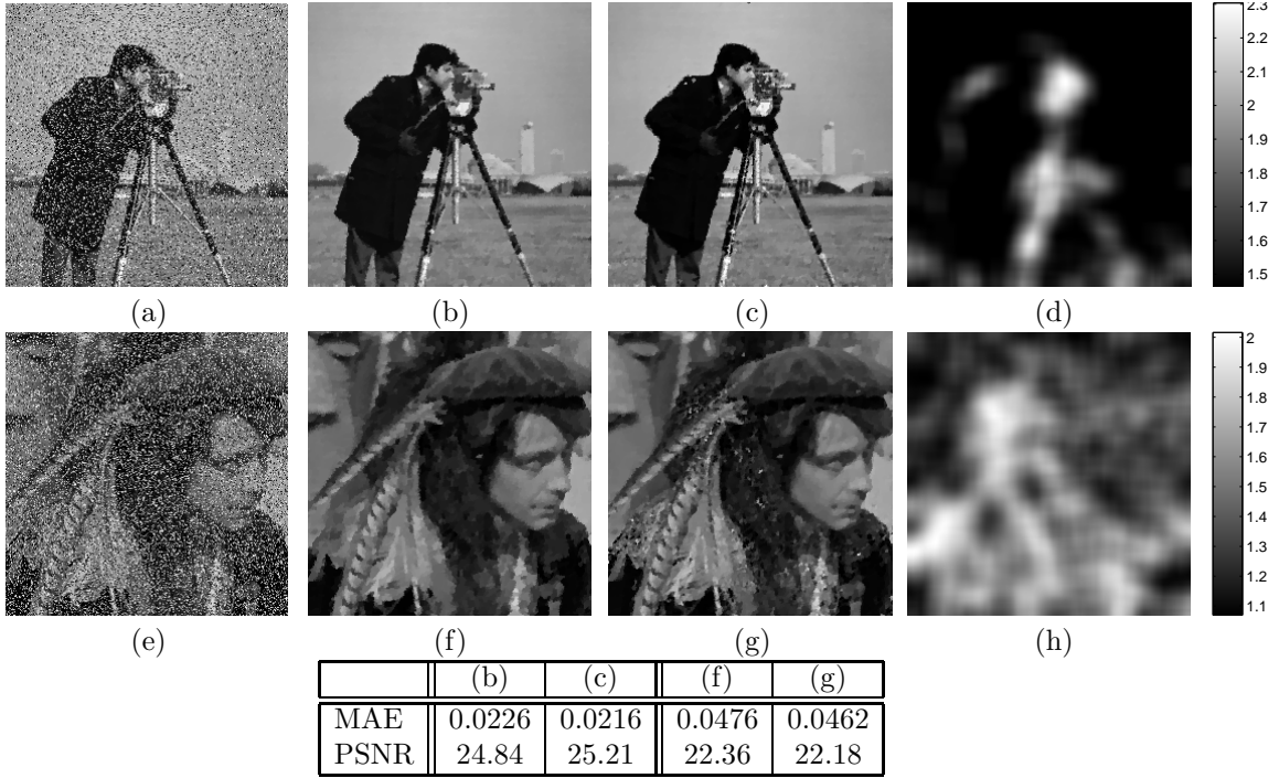
FIGURE 6. Cameraman: (a) Image with random-valued impulse noise r = 0.4 . (b) Denoising with L^1 -TV model, \lambda = 1.3 . (c) Denoising with the present method. (d) Resulting \lambda . Man: (e) Image with random-valued impulse noise r = 0.4 . (f) Denoising with L^1 -TV model, \lambda = 1.3 . (g) Denoising with the present method. (h) Resulting \lambda .
