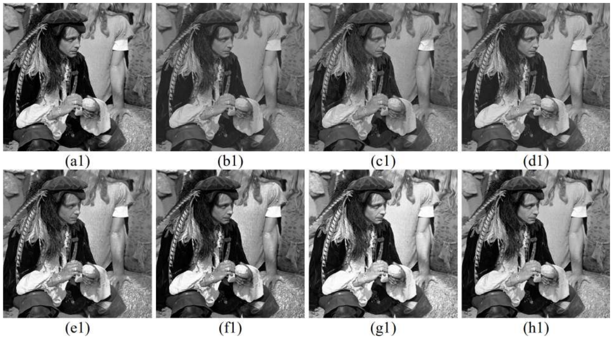
Figure 4. Processing a synthetic-degraded low-contrast image: (a1) ideal image; (b1) contrast-reduced image by (30%); the rest of the images are processed by: (c1) BPDFHE; (d1) NMHE; (e1) MMSICHE; (f1) RESIHE; (g1) DOTHE; (h1) proposed algorithm.
