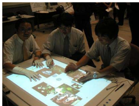
Figure 5. New furniture prototypes with larger non-sensitive areas surrounding the touch-sensitive surface.
