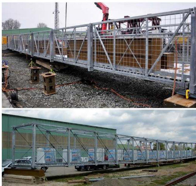
Fig. 5 full-scale testing of the “short” footbridge (on the top) and of the “long” footbridge (on the bottom)
