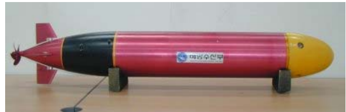
Fig. 1. Appearance of ISiMI: Torpedo-type, 2 rudders, 2 elevators, 1 propeller
