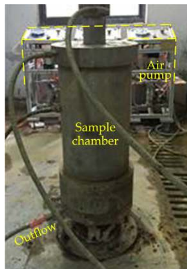
Figure 3. Principal part of the seepage test apparatus.
