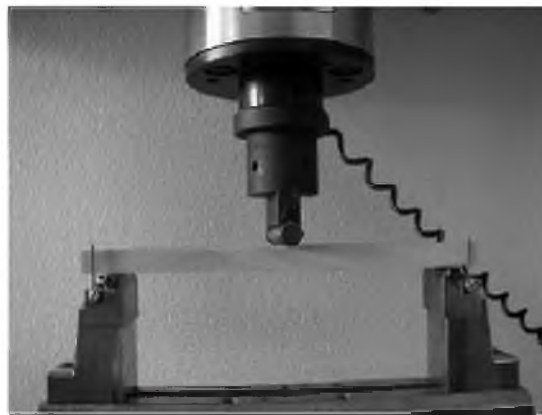
Fig. 1. Three-point bending experimental setup.
