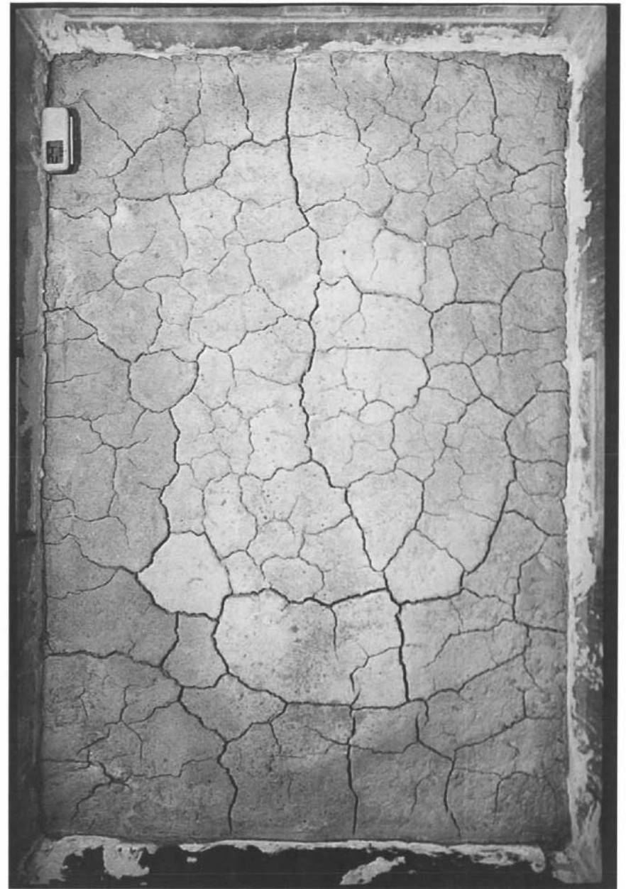
Figure 4. Aerial Photographs of the Crack Network Which Developed in Response to Desiccation – (a) Linear Cracking During a Compaction-Dry Period; and (b) Polygonal Cracking During a Wet-Dry Period.
