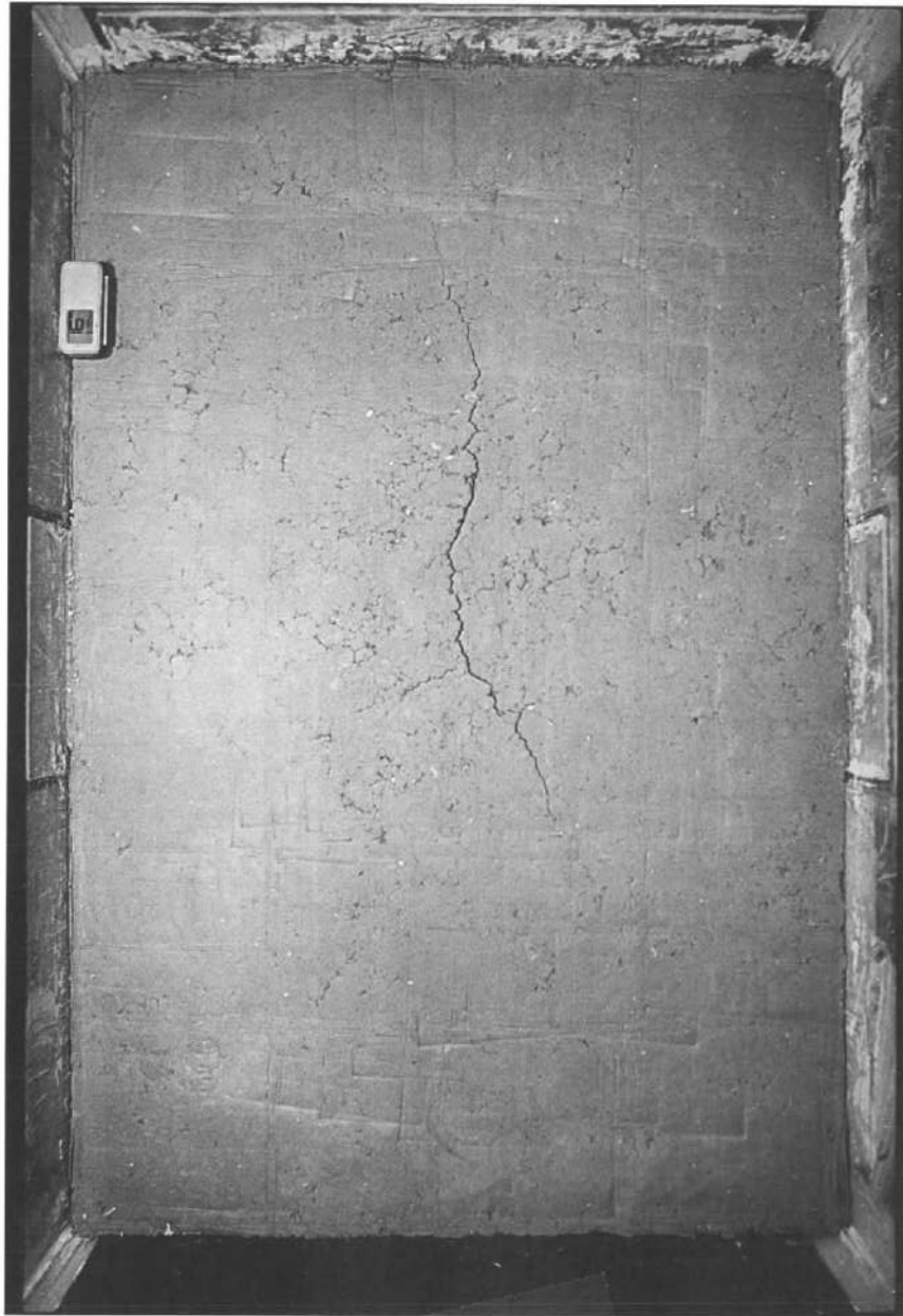
Figure 4. Aerial Photographs of the Crack Network Which Developed in Response to Desiccation – (a) Linear Cracking During a Compaction-Dry Period; and (b) Polygonal Cracking During a Wet-Dry Period.
