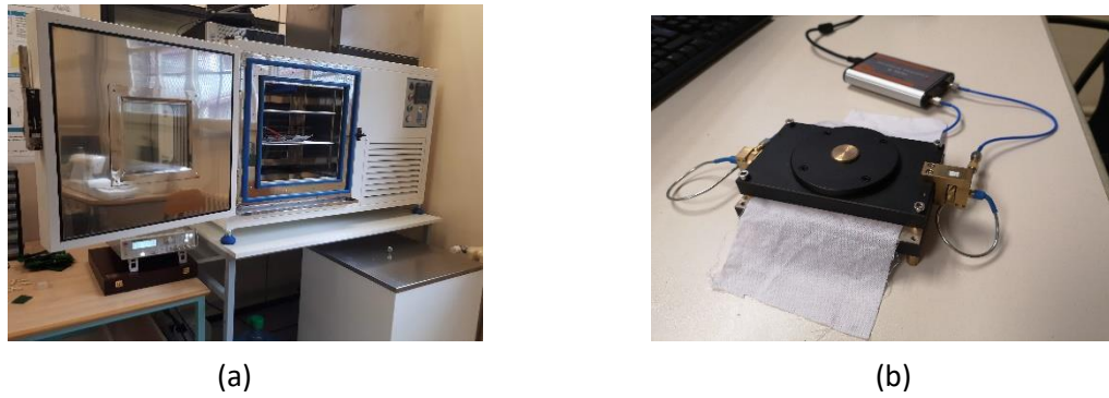
Figure 4. (a) Image of the experimental setup for humidity sensor testing. (b) Test of the permittivity and loss tangent of the textile samples based on SPDR
