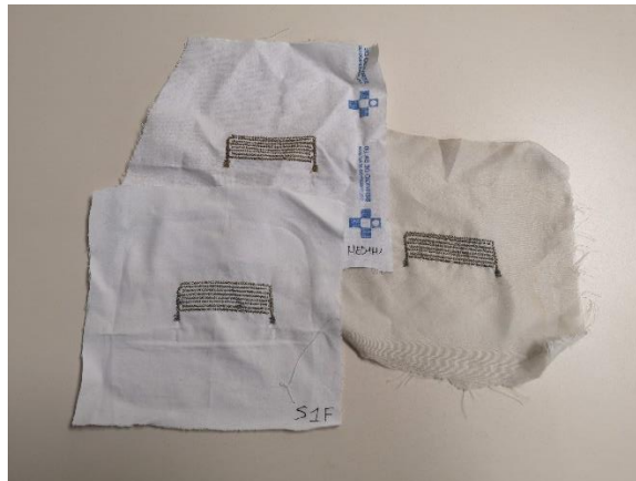
Figure 2. Sensors embroidered on different substrates. Left bottom: Cotton fabric. Left top: Medical cotton fabric. Right: Polyester fabric.
