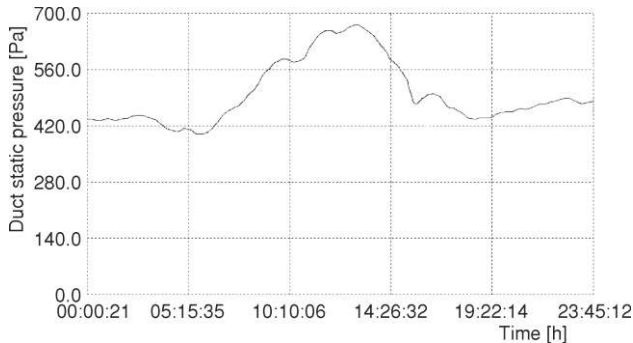
Figure 13. Variation of duct static pressure
