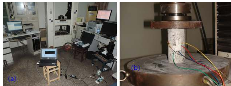
Fig 3. AGI 250 Electronic precision materials testing machine. (a) experimental devices (b) loading device.
