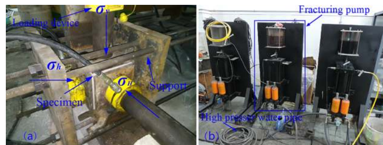
Fig 1. The physical experimental device. (a) true triaxial hydraulic fracturing system (b) fracturing fluid pump.
