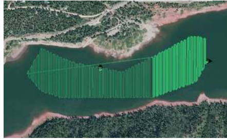
Fig. 2 The proprietary area search algorithm from Platypus generates a dense lawnmower pattern that is highly energy-inefficient.
