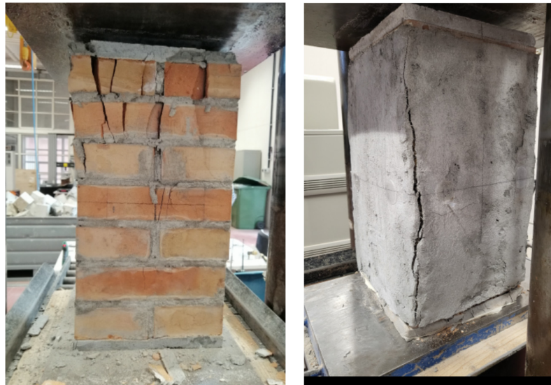
Figure 3. Unconfined and fully confined columns at failure.
