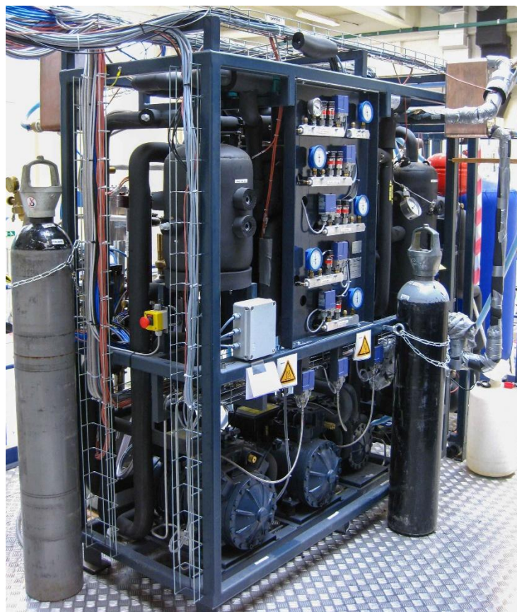
Figure 5.1: The R744 Multi-ejector refrigeration test rig.
