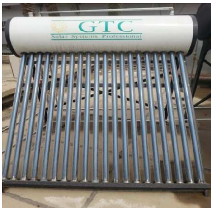
Fig 3. The experimental evacuated tube solar collector
