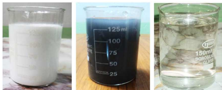
Fig 1. Show nanofluids for \text{ZrO}_2 + distilled water, Ag+ distilled water and DW
