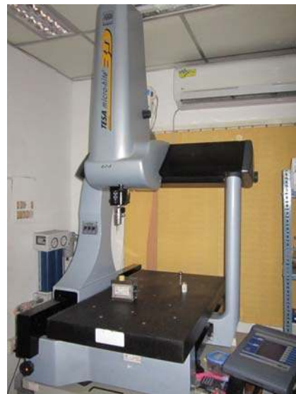
Figure 7. Photograph of CMM used for measuring ovality of drilled holes
