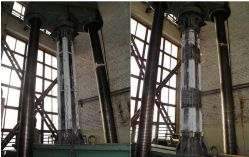
Fig. 6. The process of testing concrete columns reinforced with lamella (left) and lamellae and reinforced with holders (right)
