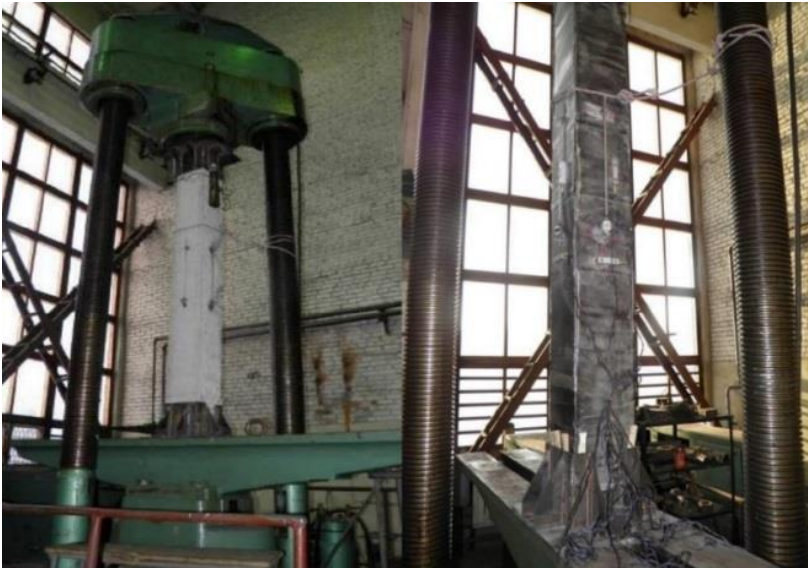
Fig. 5. The test process of unreinforced (left) and reinforced with canvases (right) concrete columns
