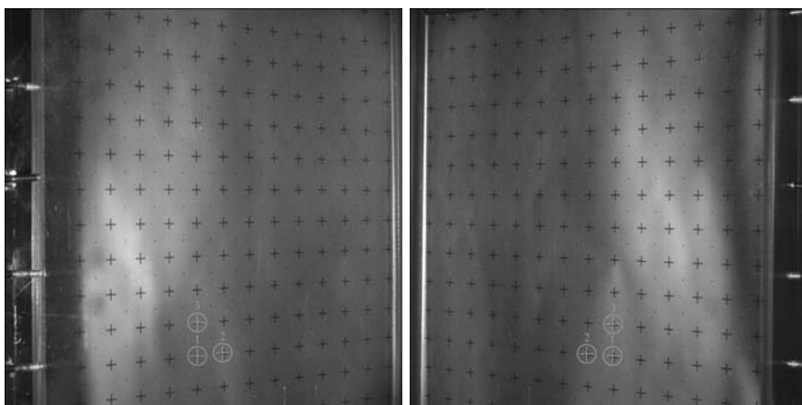
FIGURE 13. Images used for the calibration. The left image was recorded by the upper camera and the right by the lower, c.f. figure 9. The markers seen in the images are used as starting points for the marker search algorithms and for defining the world coordinates.
