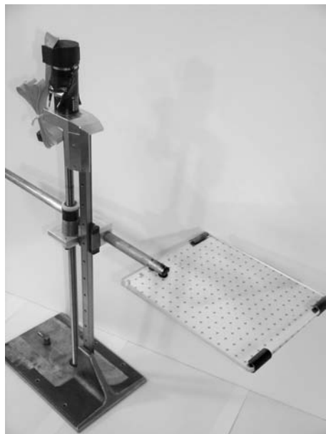
FIGURE 12. The translation stage and calibration plate setup used for the stereoscopic calibration.
