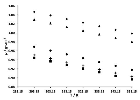
**Figure 1.** Temperature dependence of density of imidazole compounds. Circle = compound (1); square = compound (2); cross = compound (3); triangle = compound (4); diamond = compound (5).
