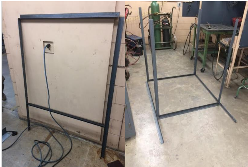
Figure 3B. Construction of angle steel frame
