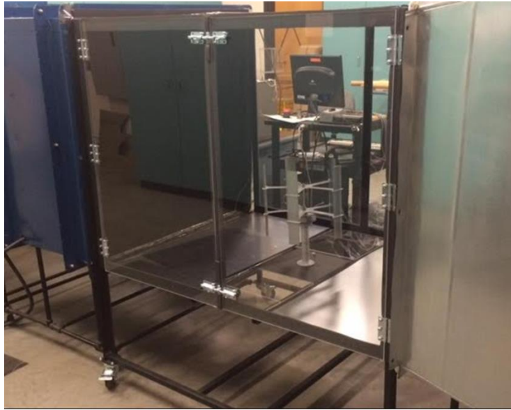
Figure 3.9. Completed assembly of new wind tunnel test section
