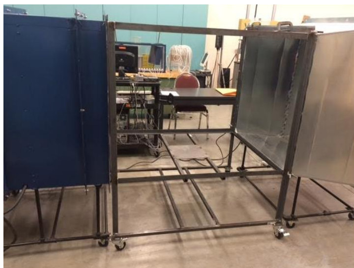
Figure 5B. New test section installed with existing wind tunnel
