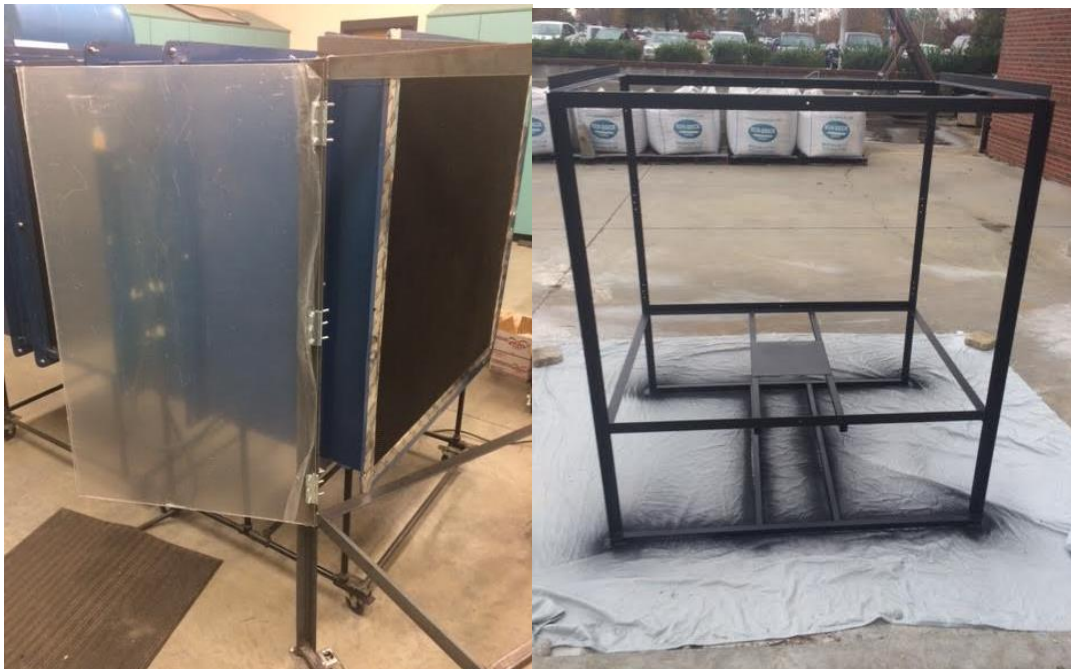
Figure 7B. Addition of clear acrylic doors (left) and painted frame (right)
