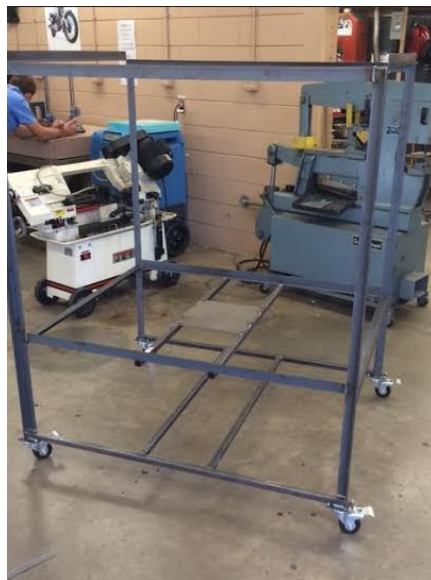
Figure 4B. Completed test section frame on casters
