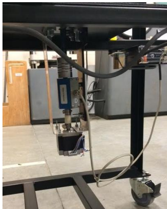
Figure 9B. Existing dynamic torque set-up with shaft, coupling, torque sensor, and generator
