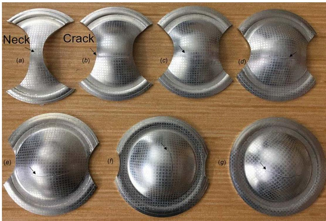
**Fig. 13** Seven deformed specimens using dome test: (a) uniaxial strain, (b) and (c) between uniaxial strain and plane–strain, (d) plane–strain, (e) and (f) between plane–strain and equibiaxial strain, and (g) equibiaxial strain deformation mode
