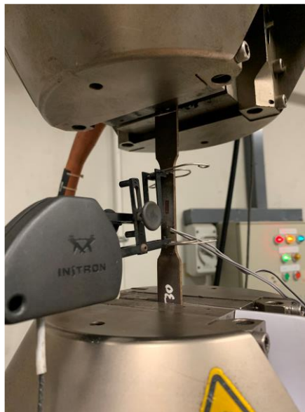
Fig. 4. Material tensile coupon test setup.
