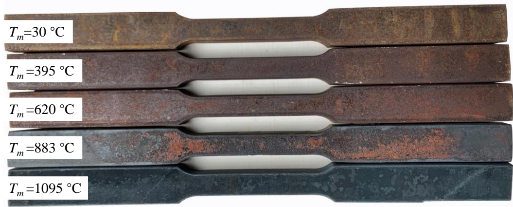
Fig. 3. Surface colours of S700 high strength steel after exposure to various levels of elevated temperature.
