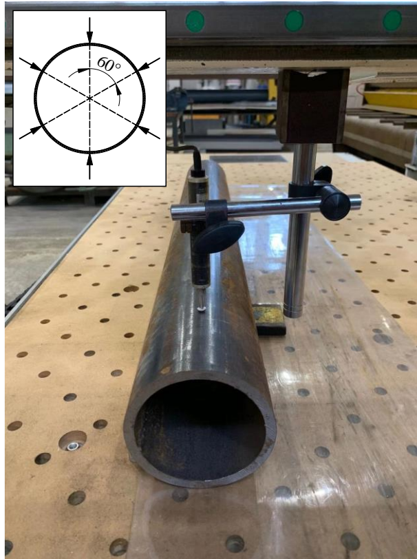
Fig. 6. Test setup for initial global geometric imperfection measurements.
