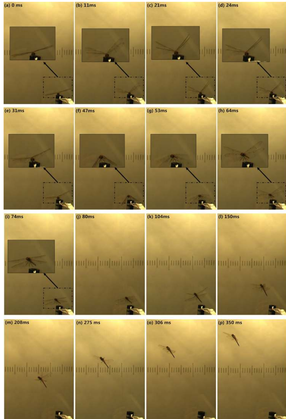
Figure 1. Video sequences (16 typical moments) of a dragonfly (D1) take-off. Two high-speed cameras are used in the experiment (the experimental scheme is detailed in the Methodology Section), and the view sequences above are from high-speed camera 2. The unit of time is ms. The vertical lines in the background are a reference scale for three-dimensional reconstruction.
