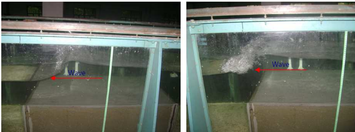
Figure 6. Wave breaking over the breakwater
