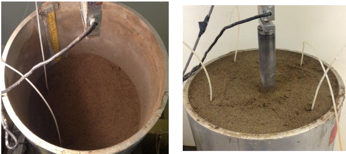
Figure 4.9 Pile installations for determination of single model pile total bearing capacity
