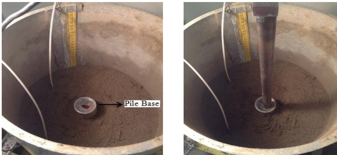
Figure 4.11 Pile installation for determination of single model pile shaft capacity
