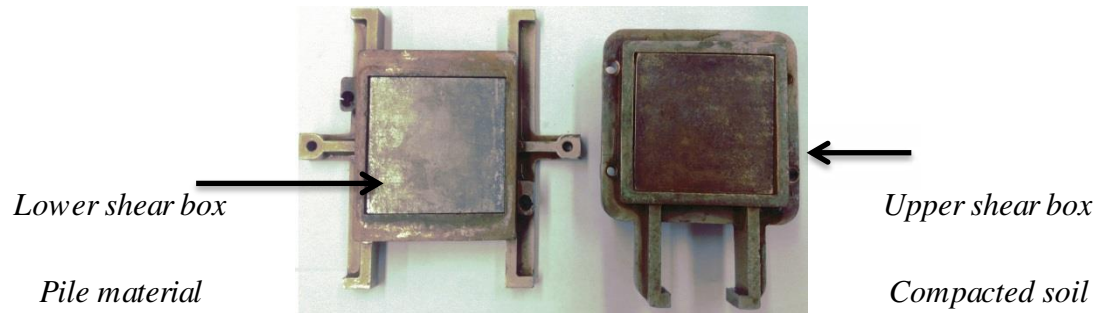
Figure 4.14 Direct shear box interface test
