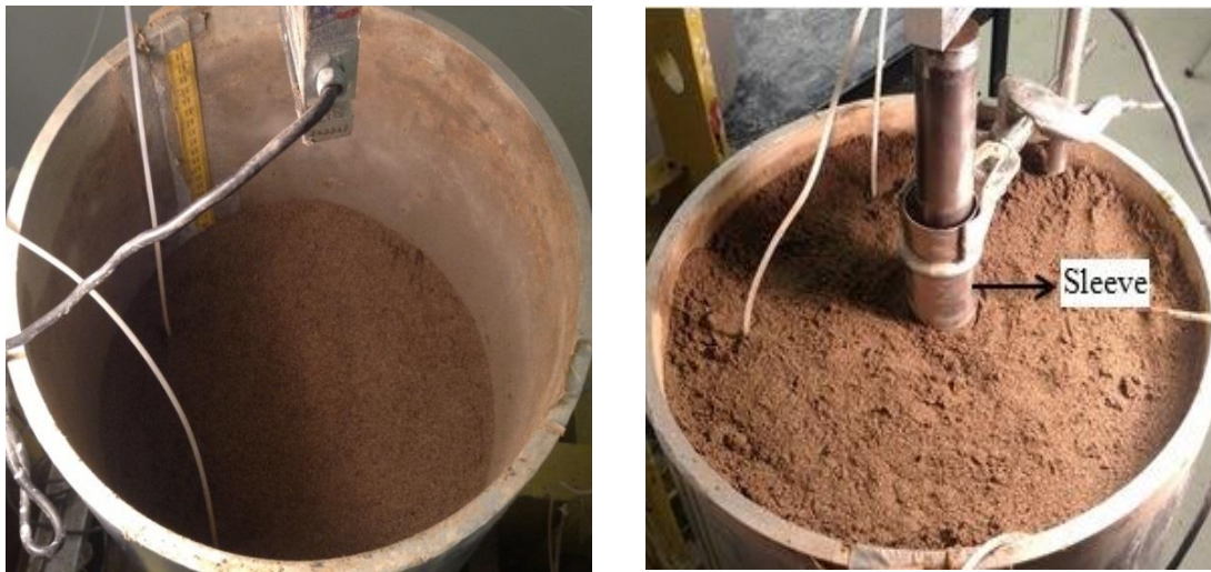
Figure 4.10 Pile installation for determination of single model pile base bearing capacity
