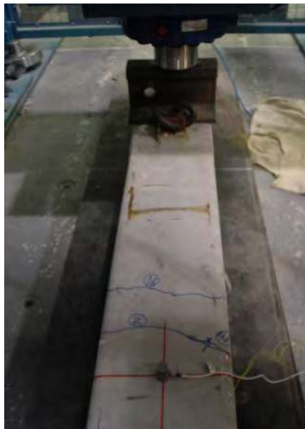
Figure 8.15 Cracks in a sleeper mid-span in soft track after 50 drops of 500 kN
