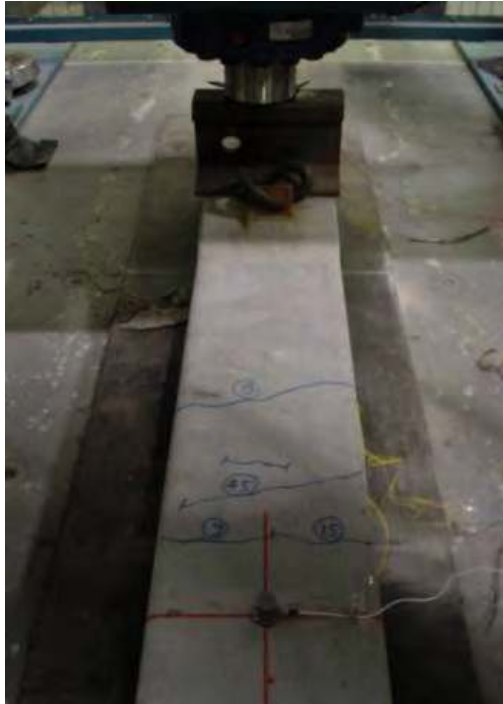
Figure 8.21 Cracks in a sleeper mid-span in hard track after 50 drops of 500 kN
