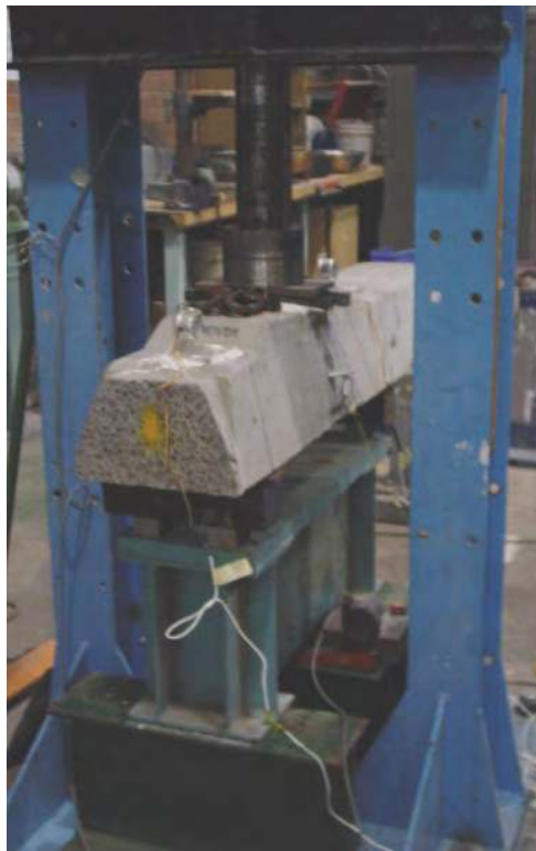
Figure 5.21 Experimental setup for rail seat- positive moment test
