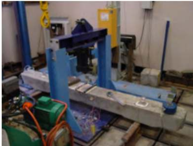
Figure 5.3 Experimental setup for centre-negative moment test
