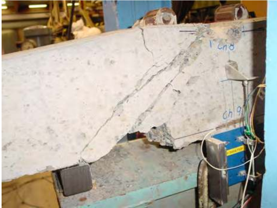
Figure 5.32 Crush and spalling along diagonal crack at rail seat
