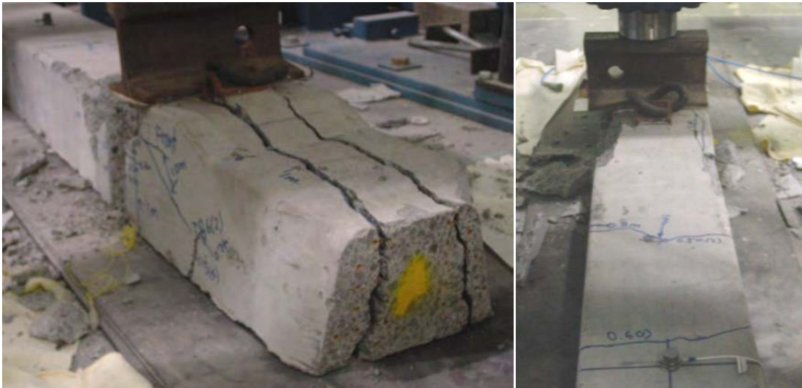
b) disintegration and top surface cracks
