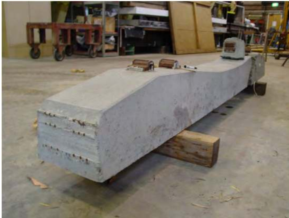
b) at another restrained rail seat (no crack found)
