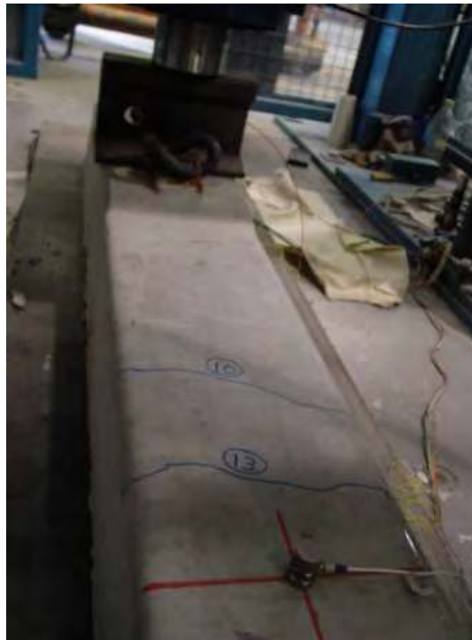
Figure 8.17 Cracks in a sleeper mid-span in soft track after 50 drops of 740 kN
