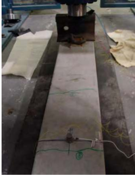
Figure 8.25 Cracks in a sleeper mid-span in hard track after 50 drops of 810 kN
