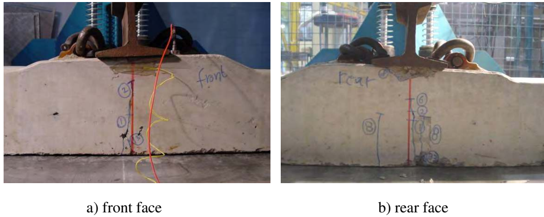
Figure 8.16 Cracks in a sleeper in soft track after 50 repeated impact of 740 kN
