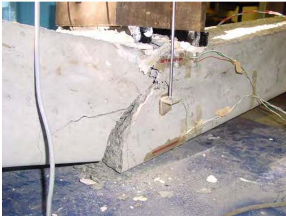
Figure 5.15 Initial flexure cracks at middle span of AUS-BG Sleeper
