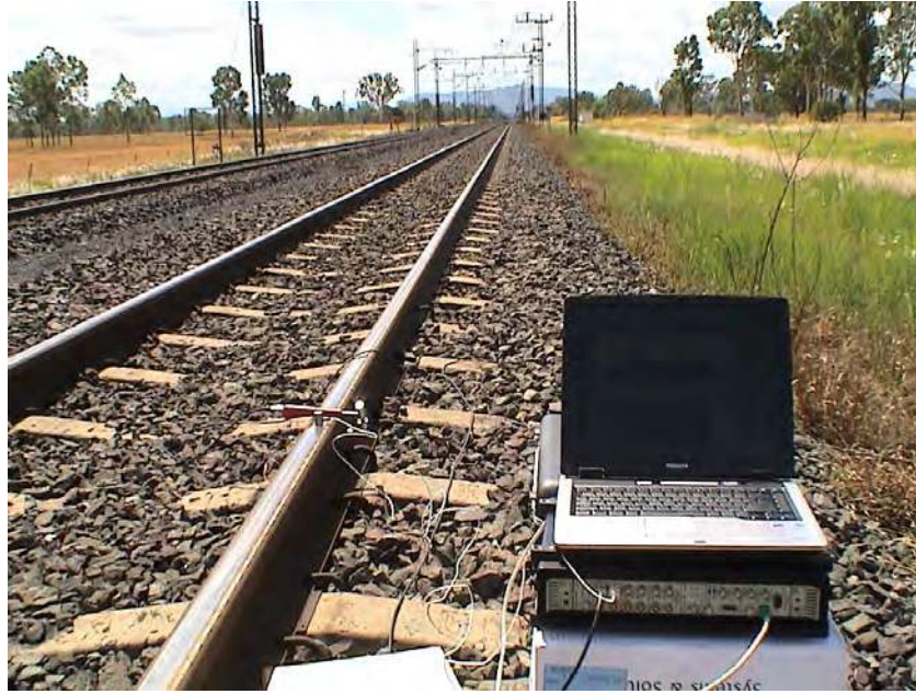
Figure 3.22 Dynamic testing installation
