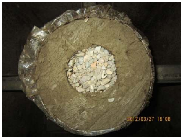
Fig. 2 Unit cell with stone column
