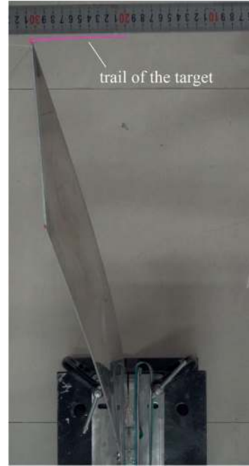
FIGURE 7: Target tracking in image plane for the wind-off experiment.
