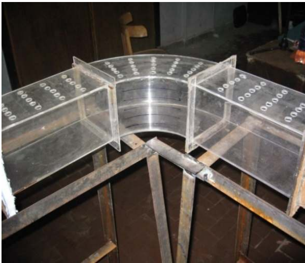
Figure 2. Perforated 90° bend and the two duct joints.
