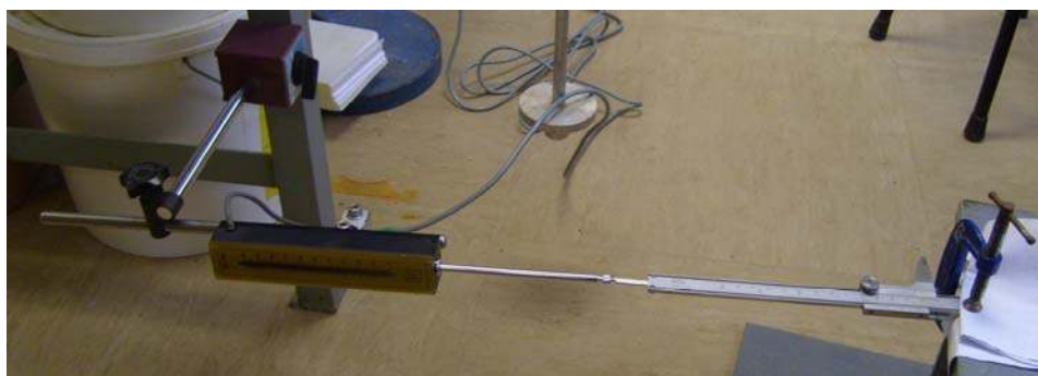
Figure 4.4 Setup for the calibration of LVDTs
