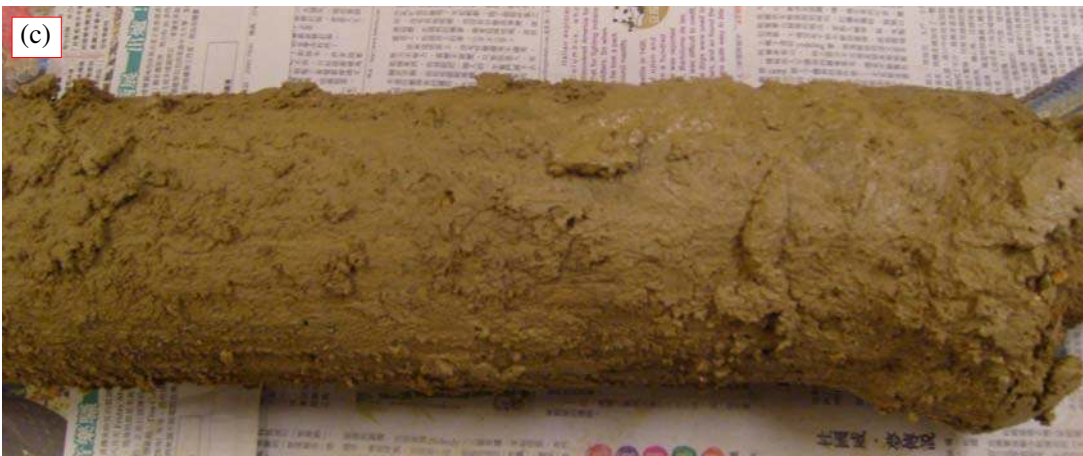
Figure 5.13 Soil nail surface near the nail head after pullout for the tests under (a) OP = 350 kPa, GP = 300 kPa, (b) OP = 240 kPa, GP = 250 kPa, and (c) OP = 80 kPa, GP = 80 kPa
