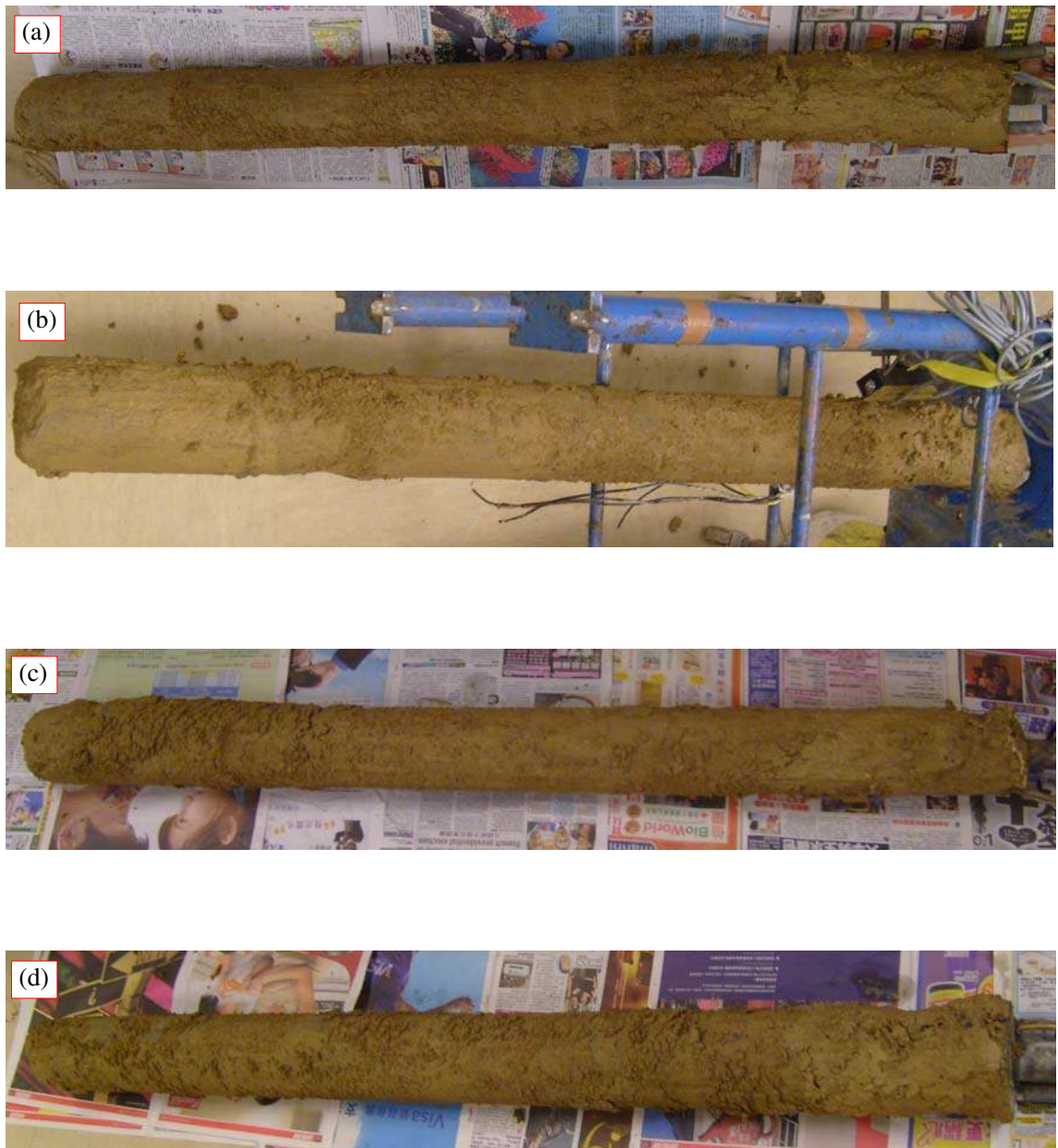
Figure 5.12 Soil nail surface after pullout for the tests under (a) OP = 350 kPa, GP = 300 kPa, (b) OP = 240 kPa, GP = 250 kPa, (c) OP = 350 kPa, GP = 130 kPa, and (d) OP = 120 kPa, GP = 80 kPa
