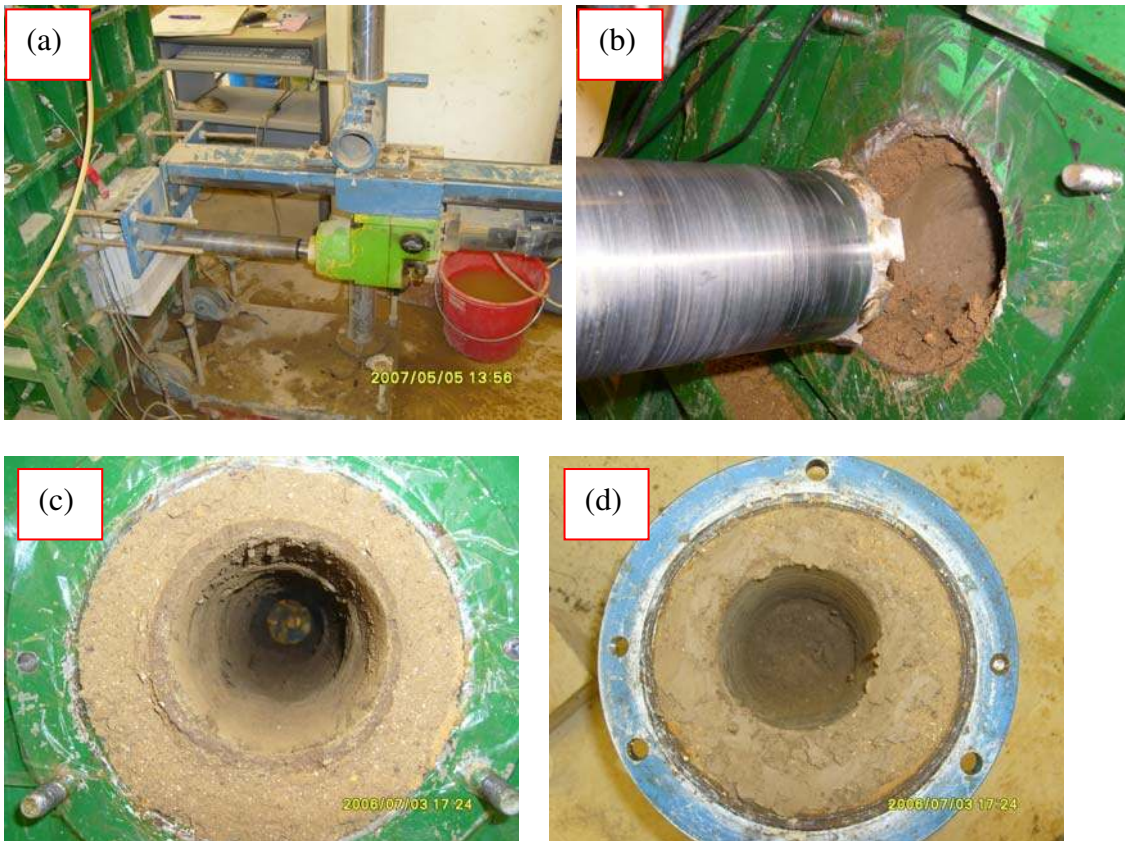
Figure 4.17 The procedure of hole drilling - (a) drilling machine, (b) during the drilling, (c) the drilled hole throughout the box, and (d) the drilled hole in the additional cylinder
