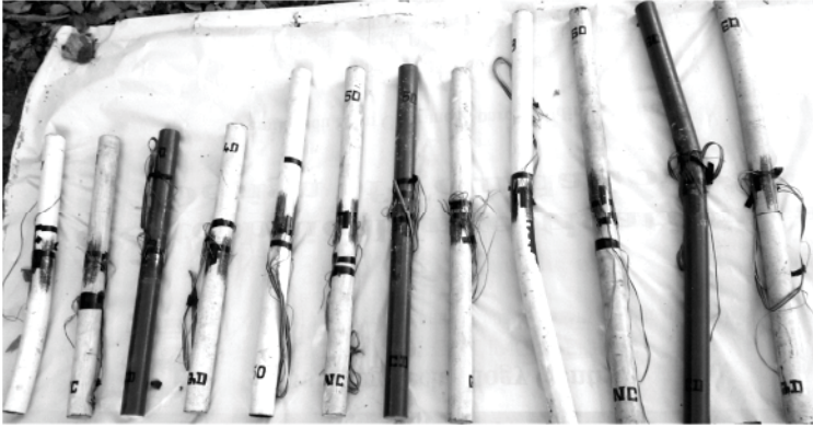
Fig. 3. Tested concrete filled tubular columns
