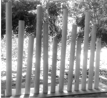
Fig. 1. Concrete filled steel tubular specimens
