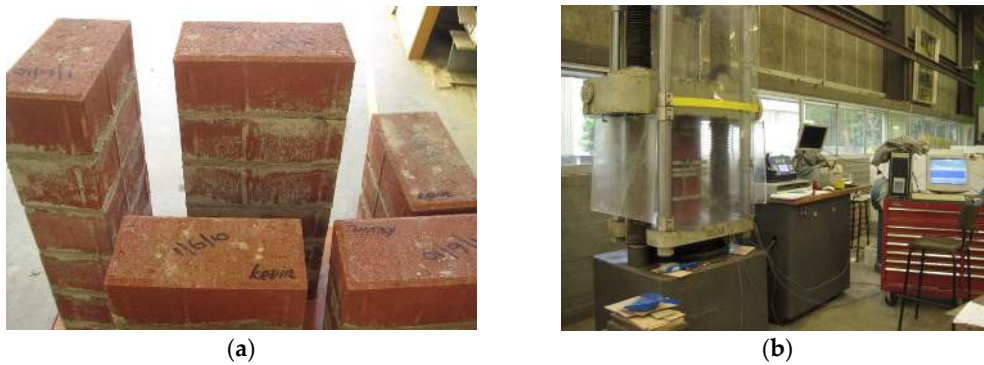
Figure 2. Photo of experimental instruments: (a) masonry prism built with mortar; (b) loading equipment.
