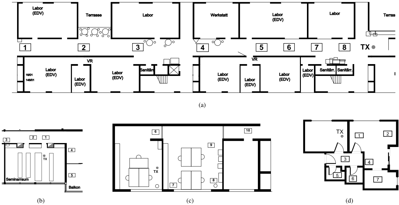
Fig. 6. Floor plans of the measured scenarios. A gray dot indicates the transmitter position, numbered rectangles indicate the receiver locations: (a) LOS, (b) and (c) office NLOS (OFF), and (d) residential NLOS (RES). Floor plans are not to scale.
