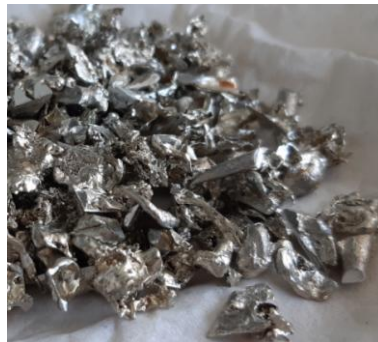
Figure 3: Granules of solid tin to be inserted in the reactor.
