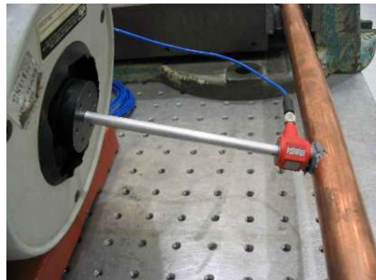
Figure 3.4. Shaker attachment for pipe example.
