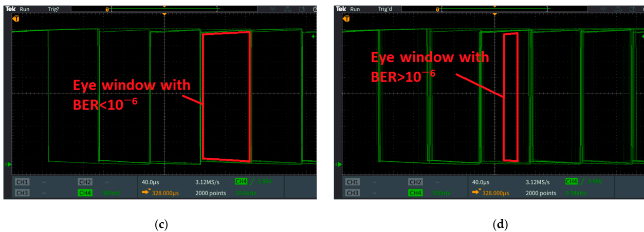
Figure 11. Eye diagrams for OOK and BFSK VLC prototypes evaluation: (a) BFSK modulation at \approx 3500 \mu\text{W}/\text{cm}^2 ; (b) BFSK modulation at \approx 3600 \mu\text{W}/\text{cm}^2 ; (c) OOK modulation at \approx 2800 \mu\text{W}/\text{cm}^2 ; (d) OOK modulation at \approx 2900 \mu\text{W}/\text{cm}^2 .
