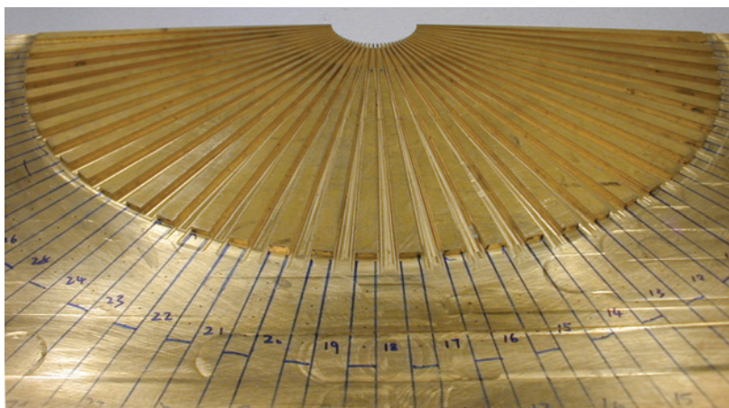
Figure 1 | Acoustic hyperlens. The lens is made of 36 brass fins (running radially from a radius of 2.7 to 21.8 cm) in air embedded on a brass substrate, spanning 180° in the angular direction. The cover sheet has been removed to expose the microstructure for this view.
