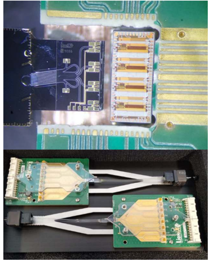
Fig. 9. Top: Photograph of a four-detector array attached to the TriPleX interposer and the four-TIA chip as well as output PCB RF lines (before wire bonding). Bottom: Two complete detector array assemblies with MPO connector, differential RF outputs and on-board TIAs.
