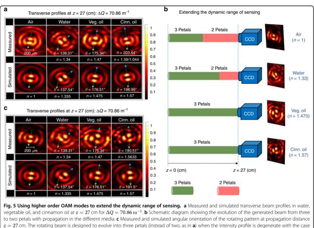
z = 27 cm. The rotating beam is designed to evolve into three petals (instead of two, as in **a**) when the intensity profile is degenerate with the case of air, thus extending the dynamic range of the sensing scheme Here, the beam is composed of OAM modes with  $\ell = 1$ , different media, the distance over which the beam
