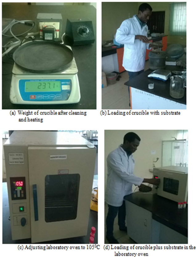
Figure 1. Experimental setup for determination of percentage total solid.
