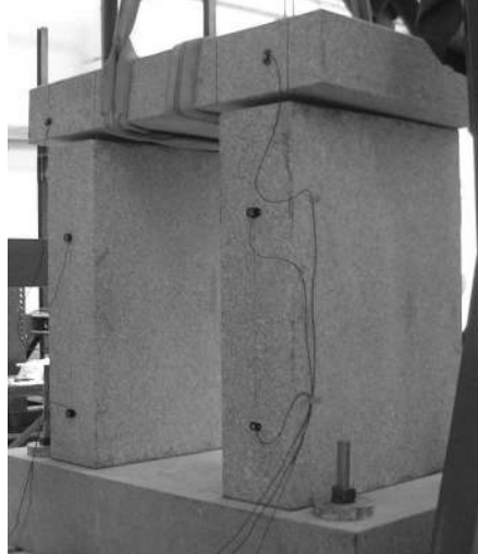
Fig. 1. Test specimens: a) Single blocks; b) Stacked blocks; c) Trilith.
