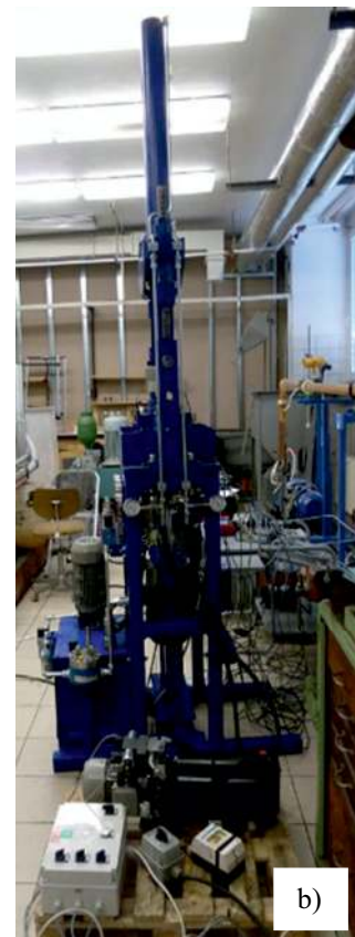
Figure 2. Experimental equipment of hydrostatic thrust bearing, a) front view, b) side view.
