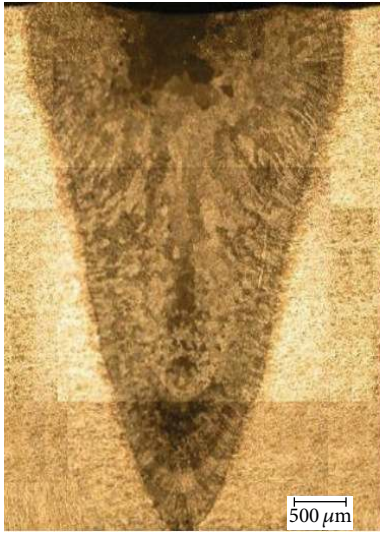
FIGURE 1: Optical macrograph of weld zones for S1.
