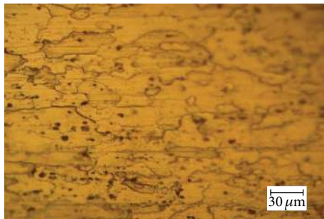
FIGURE 2: Microstructure of the parent material.
