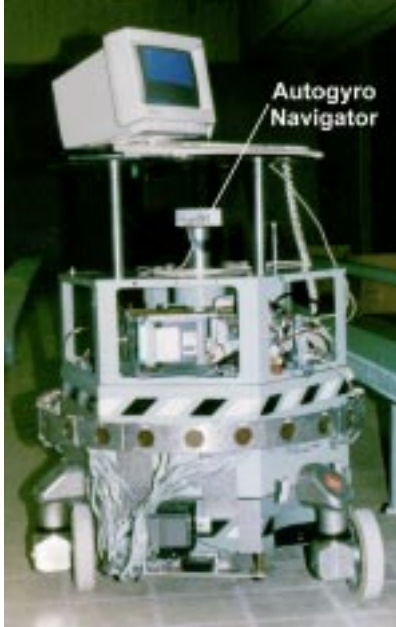
Figure 4: The University of Michigan’s mobile robot CARMEL (based on a Cybermotion K2A).
