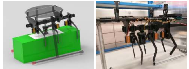
FIGURE 14. Left, rendered view of the grasping mechanism with a green brick. Right, real implementation.
