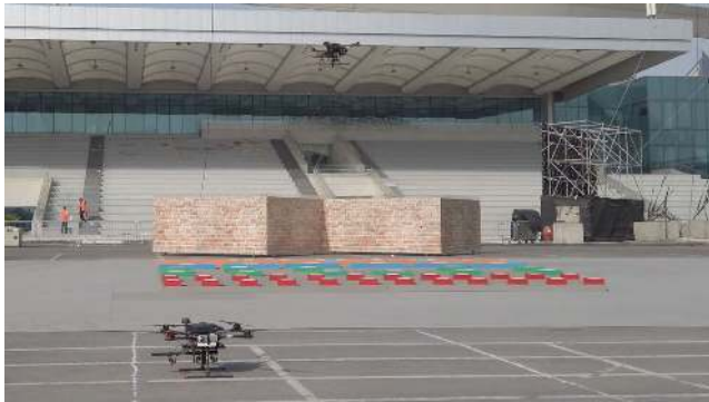
FIGURE 1. View of the arena for the MBZIRC Challenge 2. The structure to build Wall 2 has four segments, and the piles of bricks for the UAVs can be seen in front of the wall.
