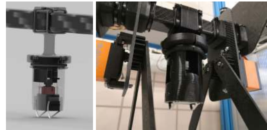
FIGURE 15. Final design integrating the Magswitch with a servomotor and the limit switches within a plastic (PLA) cylinder. Left, rendered view; right, actual implementation.
