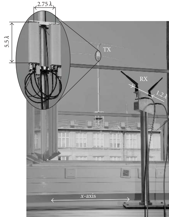
FIGURE 2: Transmit and receive antenna setups in the outdoor-to-indoor LOS scenario.
