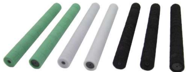
Fig. 3 Photograph of some of the cylinders (left: two cylinders covered with Regufoam Vibration 150 plus, center: two cylinders covered with Basotect, right: three cylinders covered with Regupol Vibration 550)
