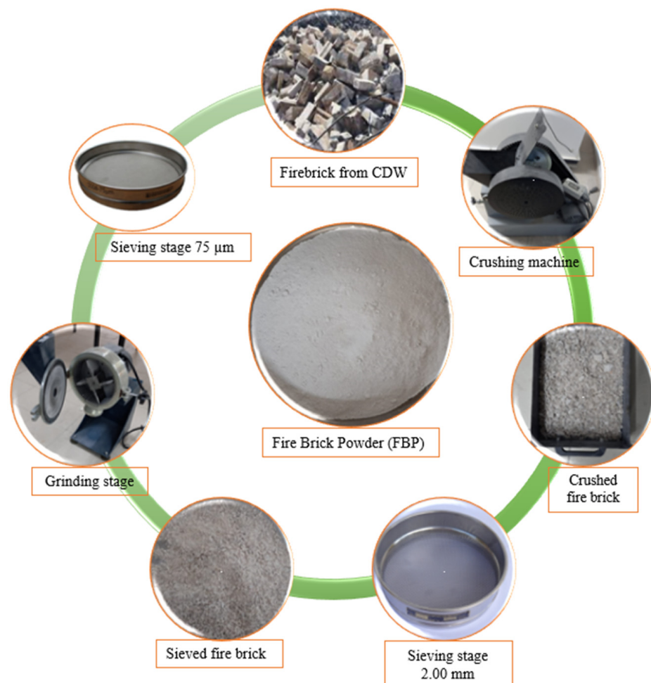
Figure 1. Production stages of firebrick powder.
