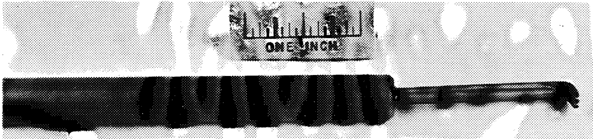
(b). - Cobra probe for sensing flow angle, total pressure and total temperature.
